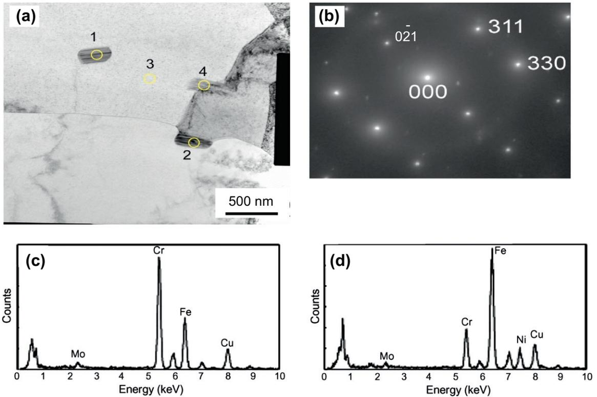
Fig. 3. TEM micrographs of banded structure; (a) bright field image [24], (b) diffraction spot from position 2, (c) EDS analysis from position 2, and (d) EDS analysis from position 3.
