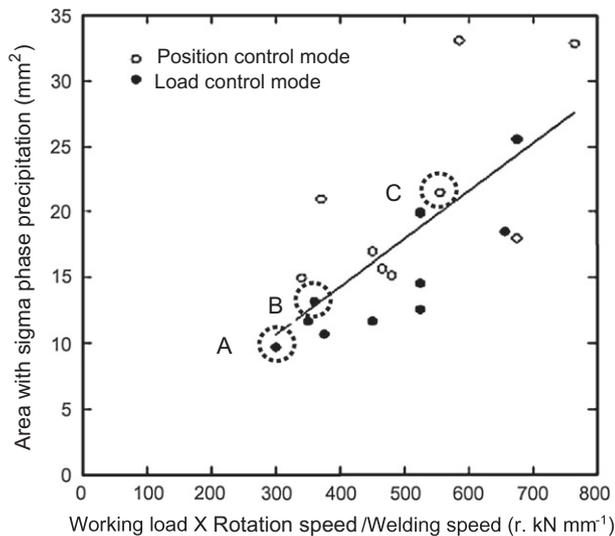
Fig. 4. The area with sigma phase precipitation as a function of heat input in both control modes.
