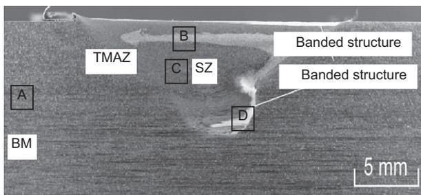
**Fig. 1.** Low-magnification overview of transversal cross-section of a typical friction stir welding zone (30 kN, 5 rad s<sup>-1</sup>, 20 mm min<sup>-1</sup>) [24].
