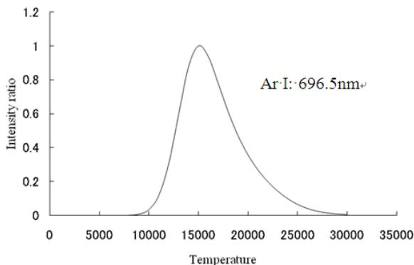
Fig.4 Relationship between temperature and intensity ratio at 696.5nm (Ar I).
