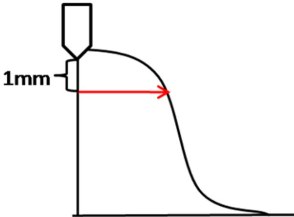
Fig.6 Position where the radial temperature distribution shown in Fig. 7 was measured.
