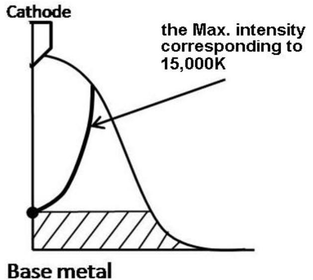
Fig.5 Concept of inversion from the intensity to the temperature.
