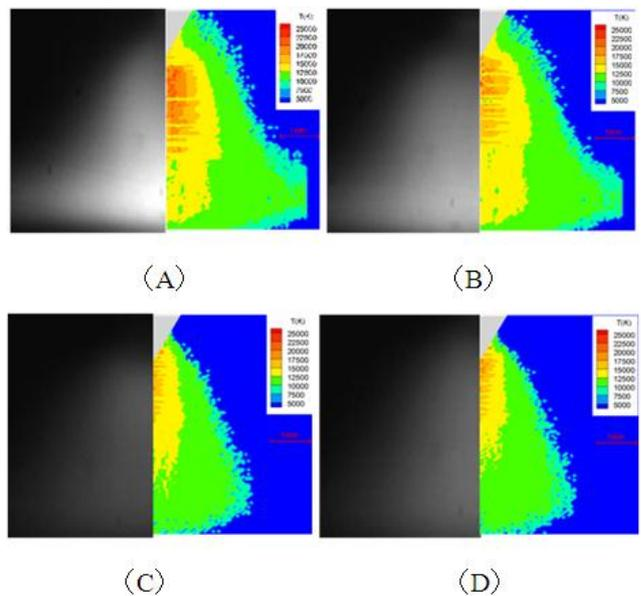
Fig.11 Time variation of temperature distributions of TIG pulsed arc at the times (A) ~ (D) marked in Fig. 10.
