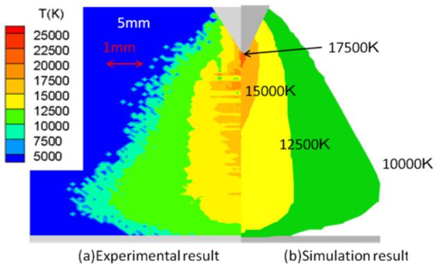
Fig.8 (a) Experimental result and (b) simulation result of two-dimensional temperature distributions.
