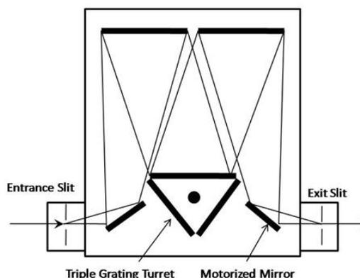
Fig.2 Schematic diagram of monochromator.
