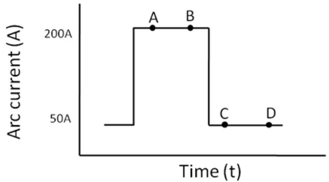
Fig.10 Current waveform of TIG pulsed arc.
