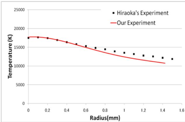
Fig.7 Temperature distributions in radial direction below 1mm from cathode tip.
