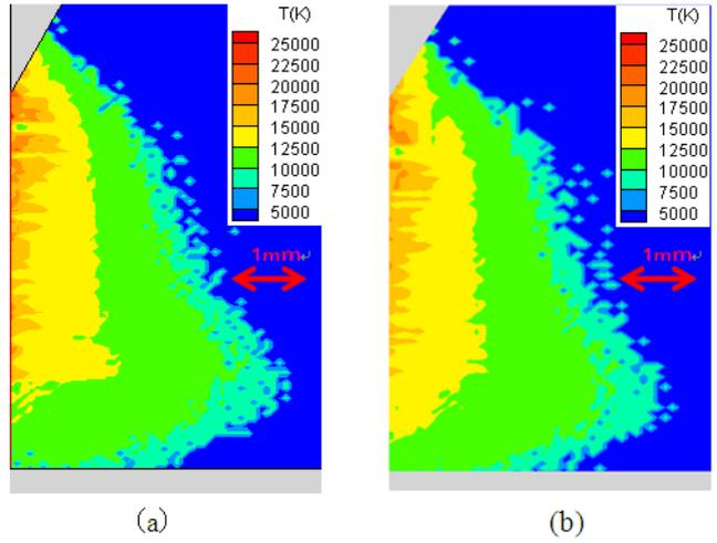
Fig.9 Comparison of temperature distributions between cases of conical tip of (a) 45°and (b) 60°.
