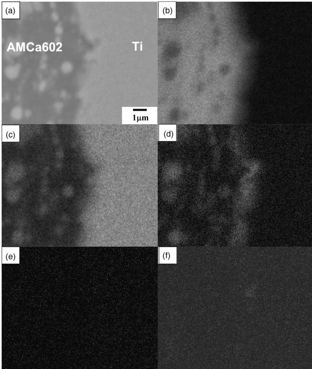
Fig. 3. SEM image (a) and characteristic X-ray images of Mg (b), Ti (c), Al (d), Mn (e) and Ca (f) near joint interfaces of titanium and AMCa602.
