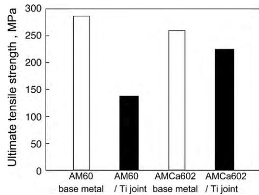
Fig. 5. Tensile strengths of FSW joints of titanium and magnesium alloys.
