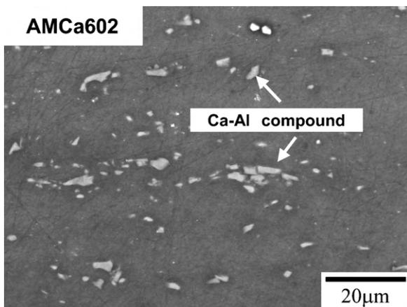
Fig. 4. SEM image of AMCa602 base metal.
