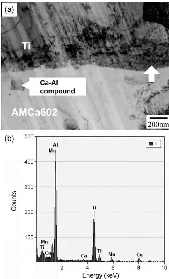
**Fig. 6.** TEM observation result of the joint interface of titanium and AMCa602 joint: (a) bright field image and (b) EDX spectrum from the spot indicated by the arrow (a).
