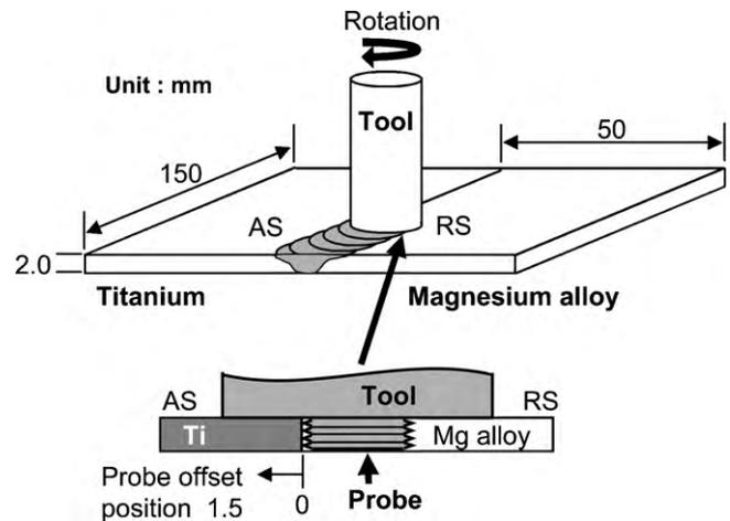
**Fig. 1.** Schematic illustration of joint arrangement in FSW.
