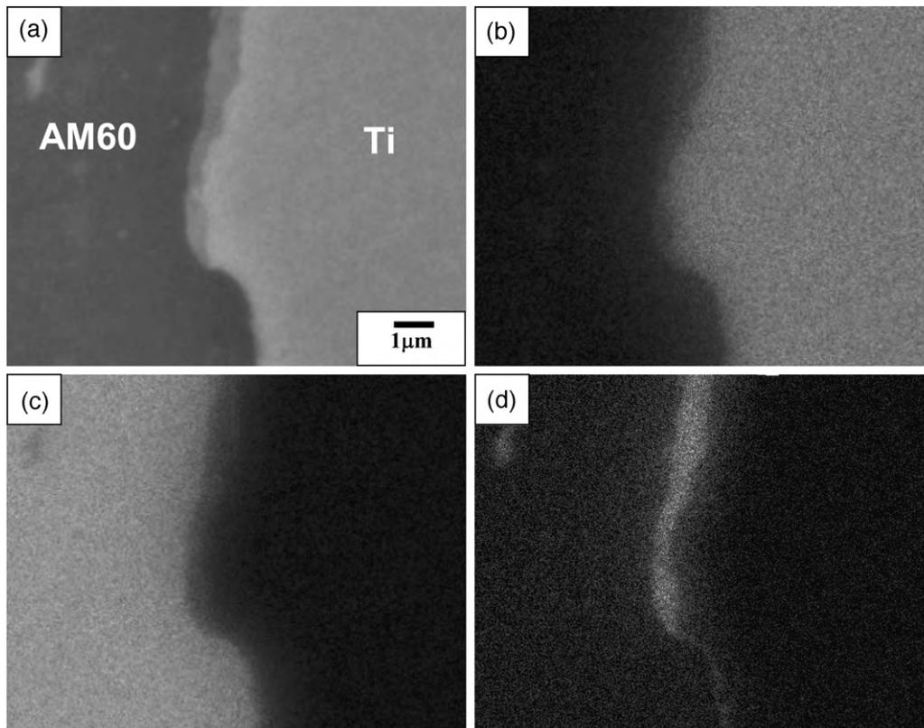
**Fig. 2.** SEM image (a) and characteristic X-ray images of Ti (b), Mg (c) and Al (d) near joint interfaces of titanium and AM60.
