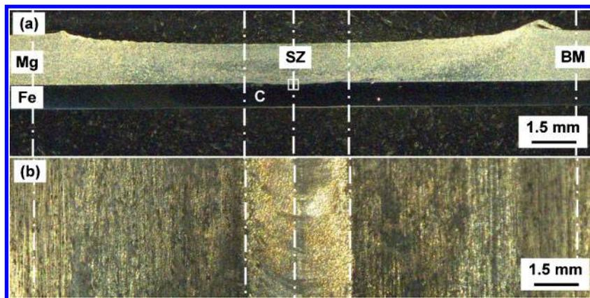
2 a cross-sections of brushed finish steel joint and b front view of fracture surface at Mg alloy side; image shown are from fractured weld samples taken from top surface of bottom Mg sheet
