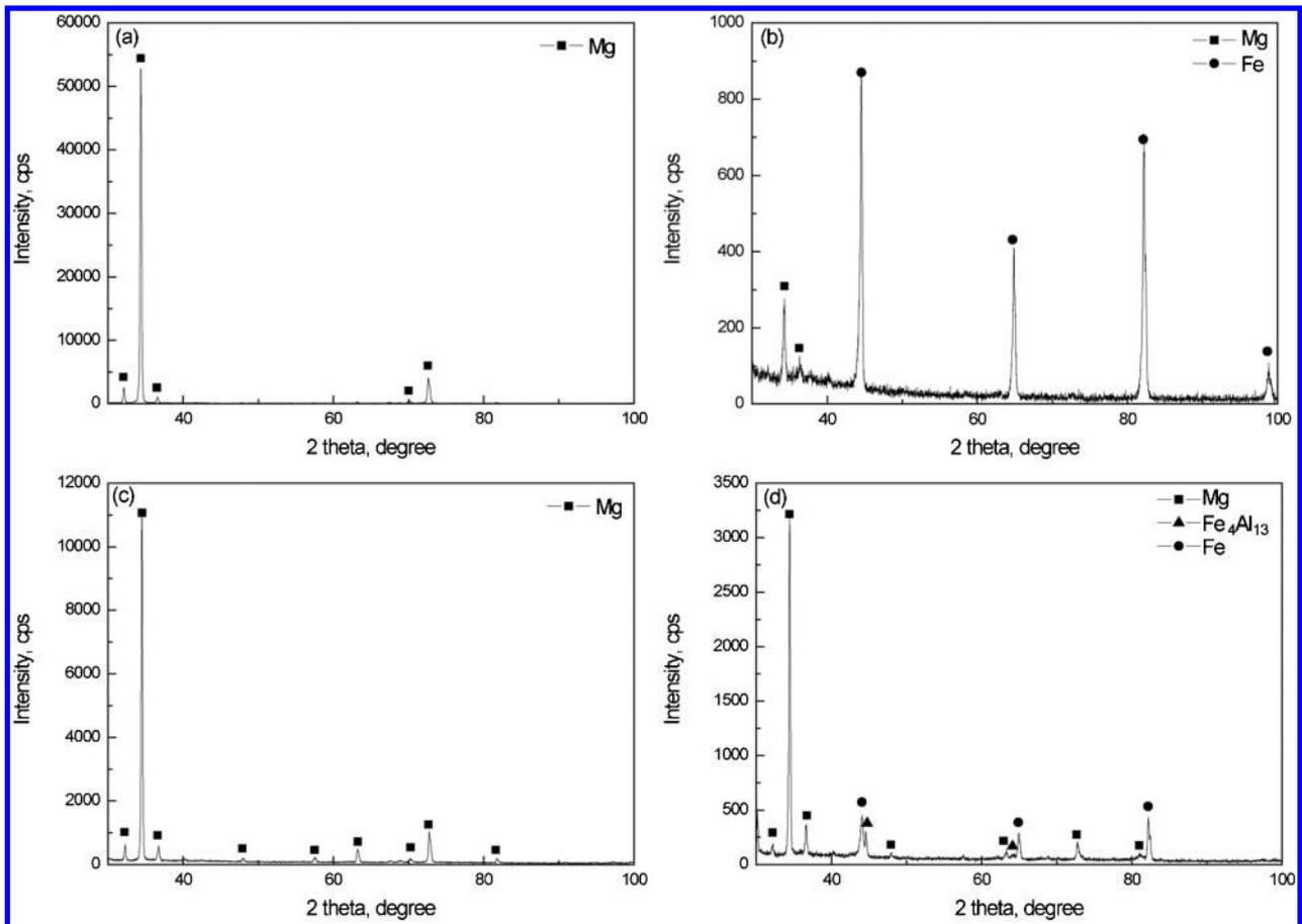
6 X-ray diffraction analysis results from fracture surface of joints ( $3.33 \text{ mm s}^{-1}$ ) a from Mg side of brushed finish steel joint; b from Fe side of brushed finish steel joint; c from Mg side of zinc coated steel joint and d from Fe side of zinc coated steel joint
