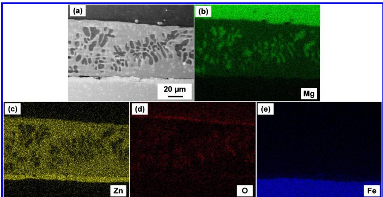
4 SEM and EDS analysis results at position B shown in Fig. 1a
