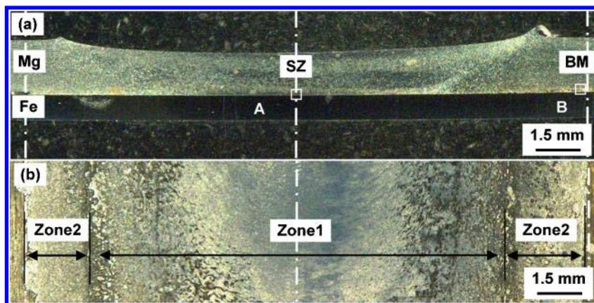
1 a cross-sections of zinc coated steel joint and b front view of fracture surface at Mg alloy side; image shown are from fractured weld samples taken from top surface of bottom Mg sheet
