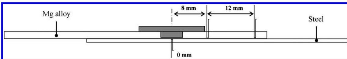
7 Locations of inserted thermocouples for temperature measurement during FSW ( $3\cdot33\text{ mm s}^{-1}$ )
