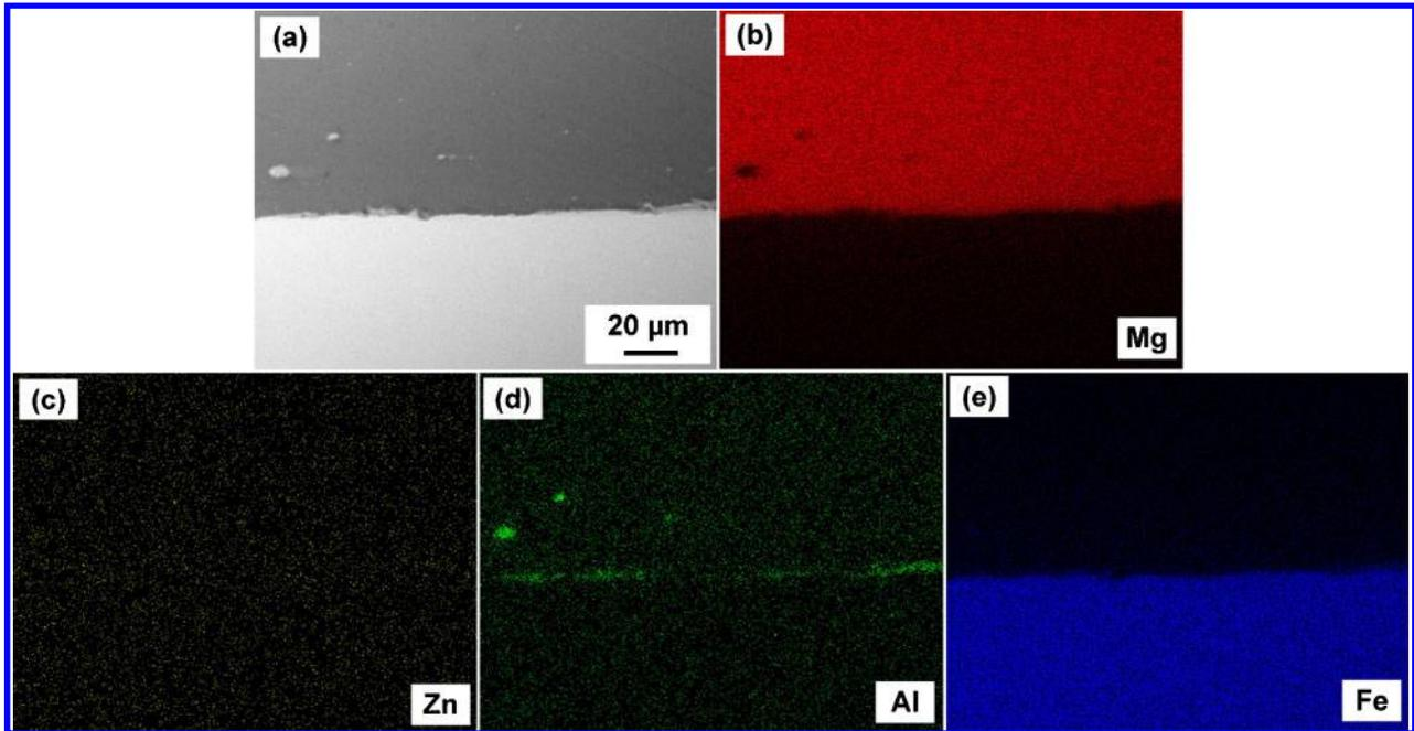
3 SEM and EDS analysis results at position A shown in Fig. 1a
