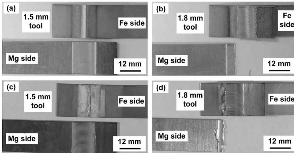
Fig. 3. Effect of tool geometries on the fracture locations of the joints: (a, b) brush finished steel joints; (c, d) zinc coated steel joints.
