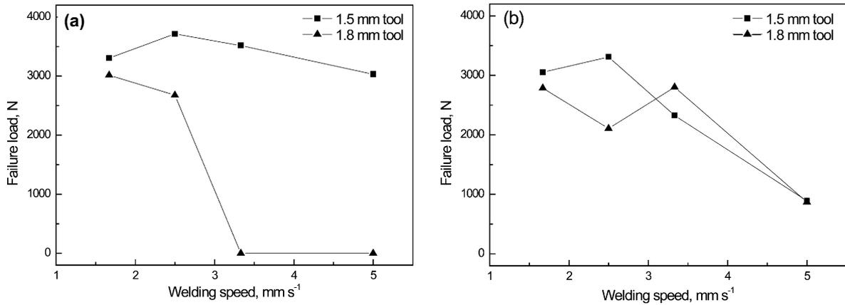
Fig. 2. Effect of tool geometries on the tensile strength of the joints: (a) brush finished steel joints; (b) zinc coated steel joints.
