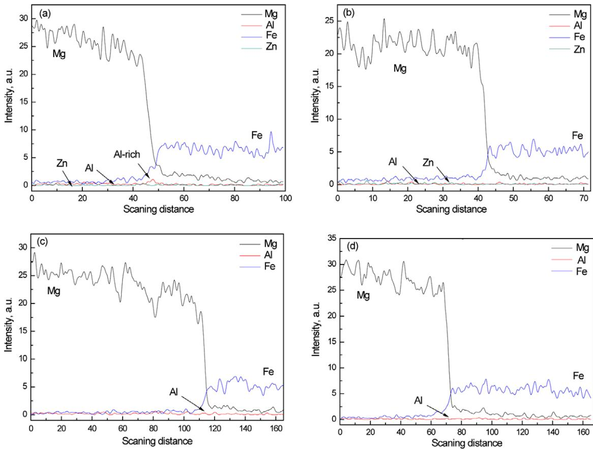
Fig. 8. EDS analysis results along the scan lines shown in Fig. 7: (a) along the scan line shown in Fig. 7a; (b) along the scan line shown in Fig. 7b; (c) along the scan line shown in Fig. 7c and (d) along the scan line shown in Fig. 7d.
