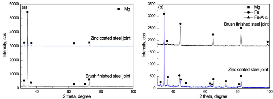
**Fig. 9.** XRD analysis results from the fracture surface of the joints welded using 1.5-mm-length probe ( $3.33 \text{ mm s}^{-1}$ ): (a) from Mg side of the joints and (b) from Fe side of the joints.
