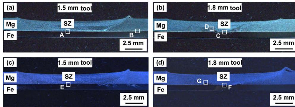
Fig. 4. Cross-sections of the joints: (a, b) zinc coated steel joints; (c, d) brush finished steel joints.
