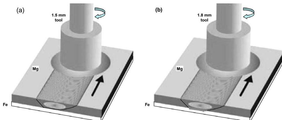
**Fig. 1.** A graphic scheme of the FSW process.
