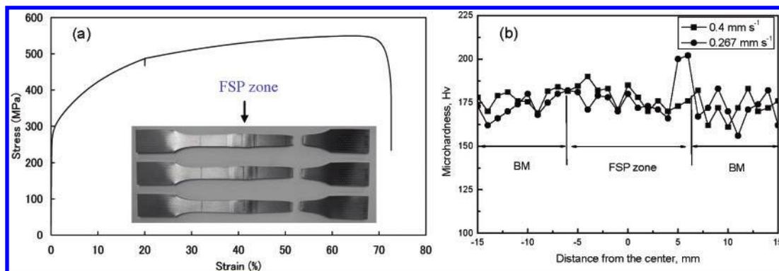
a typical stress–strain curve; b microhardness distribution of FSP zone ( $5 \text{ rad s}^{-1}$ )
