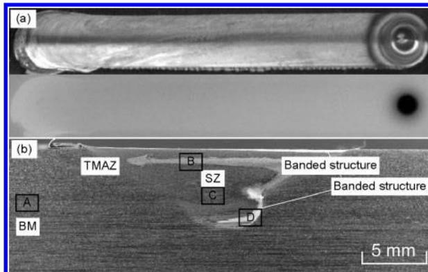
a appearance of FSP zone and X-ray inspection result;
