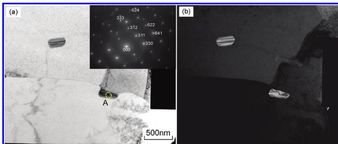
a bright field image; b dark field image from diffraction spot [311]
