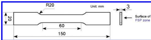
1 Schematic of tensile test specimen
