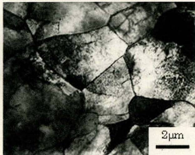
Figure 3 – TEM bright field images of stir zones of IF steel welded at 400 mm/min
