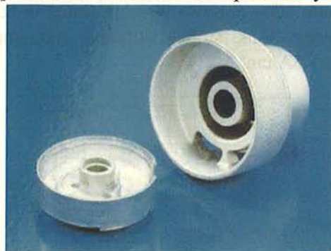
Fig. 10 Application of laser alloying for tape deck cylinder manufactured by aluminum alloy.
