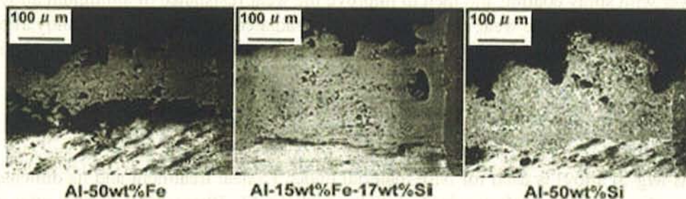
Fig. 2 Cross section view of sprayed layers.
