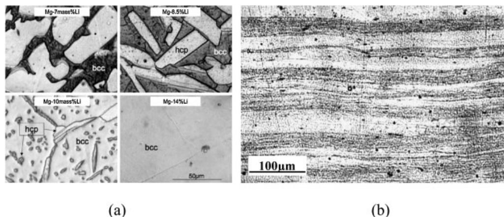
■ Figure 1. Microstructure of Mg-Li alloy (a) and cold-rolled Mg-14 wt.-% Li alloy (b).
