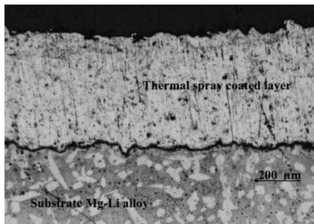
Figure 2. Example of cross-section view of plasma thermal sprayed surface.
