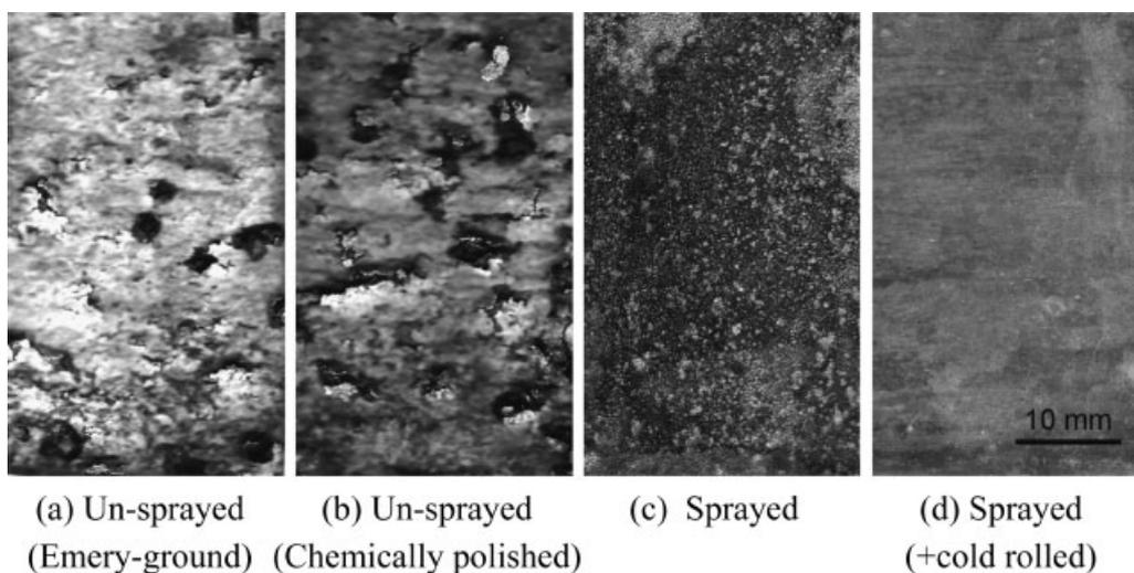
■ Figure 3. Surfaces after corrosion test (test duration: 24 h).
