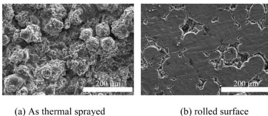
■ Figure 4. Features of surface: (a) as sprayed, (b) cold-rolled 3%.
