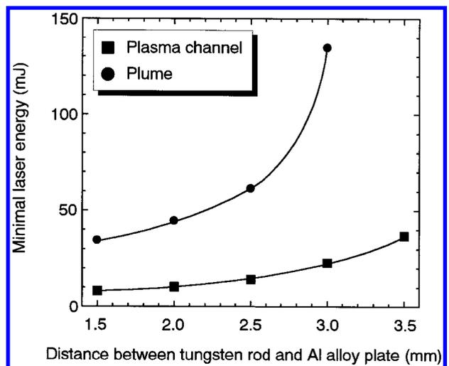
**3 Minimum laser energies required to trigger arc discharge using plasma channel and plume methods, as function of distance between tungsten rod and aluminium alloy plate**
