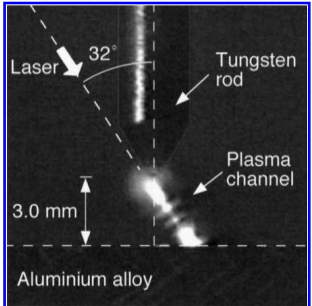
**2 Plasma channel between tungsten rod and aluminium alloy plate in argon gas, produced by pulsed laser focusing at laser energy of 23 mJ (optical)**
