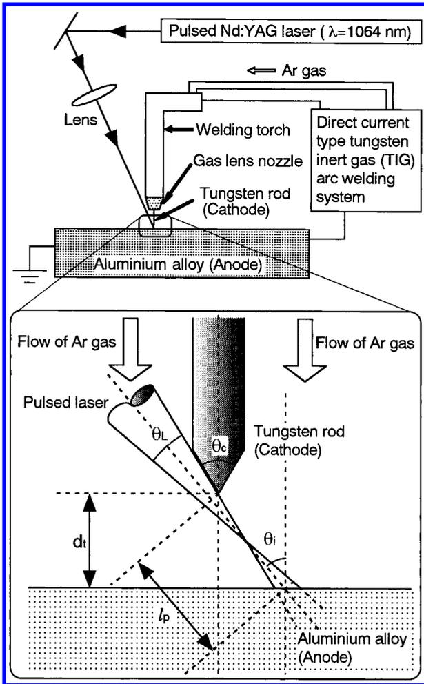
**1 Schematic diagram of experimental configuration for triggering arc discharge, employing direct current tungsten inert gas arc welding system and pulsed Nd:YAG laser: cathode and anode of system consisted of tungsten rod and aluminium alloy plate, respectively, and laser beam was focused into argon gas ejected from nozzle between electrodes by lens of 150 mm focal length at incident angle of 32°**
