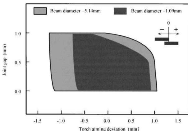
9 Effect of laser beam diameter on tolerance of joint gap (wire feedrate  $13 \text{ m min}^{-1}$ , welding current 135 A, arc voltage 16.8 V, EN ratio 30%, laser power 2.0 kW, and welding speed  $4 \text{ m min}^{-1}$ )
