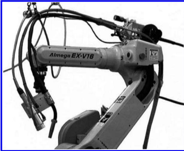
1 Laser assisted alternating current (ac) pulsed metal inert gas (MIG) welding system
