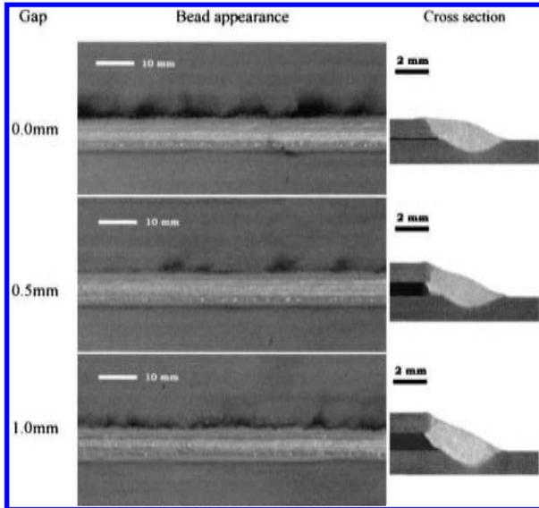
5 Effect of joint gap on bead appearance and cross-section (optical) for laser assisted ac pulsed MIG welding at speed of  $4 \text{ m min}^{-1}$  (wire feedrate  $13 \text{ m min}^{-1}$ , welding current 135 A, arc voltage 16.9 V, EN ratio 30%, and laser power 2.5 kW)
