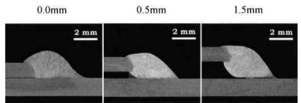
4 Effect of joint gap on cross-sections (optical) obtained for ac pulsed MIG arc welding at speed of  $3 \text{ m min}^{-1}$  (wire feedrate  $12 \text{ m min}^{-1}$ , welding current 130 A, arc voltage 16.6 V, and electrode negative (EN) ratio 30%)
