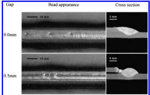
2 Effect of joint gap on bead appearance and cross-section (optical) for direct current (dc) pulsed MIG arc welding at speed of  $4 \text{ m min}^{-1}$  (wire feedrate  $13 \text{ m min}^{-1}$ , welding current 215 A, and arc voltage 19–8 V)
