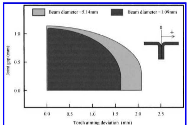
10 Effect of laser beam diameter on tolerances of joint gap and deviations in torch aim for flare joint configuration (wire feedrate  $14 \text{ m min}^{-1}$ , welding current 150 A, arc voltage 17.2 V, EN ratio 30%, laser power 1.5 kW, and welding speed  $4 \text{ m min}^{-1}$ )
