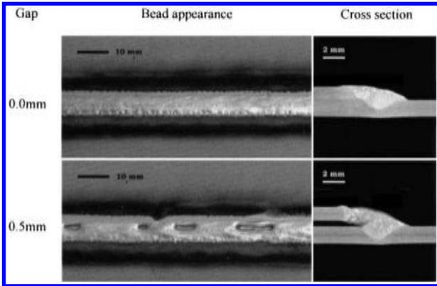
3 Effect of joint gap on bead appearance and cross-section (optical) for dc pulsed MIG arc and laser beam hybrid welding at speed of  $4 \text{ m min}^{-1}$  (wire feedrate  $8.5 \text{ m min}^{-1}$ , welding current 135 A, arc voltage 17.1 V, and laser power 2 kW)
