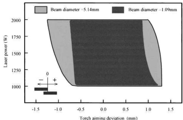
7 Effect of laser beam diameter on tolerance of deviations in torch aim (wire feedrate  $13 \text{ m min}^{-1}$ , welding current 135 A, arc voltage 16.8 V, EN ratio 30%, and welding speed  $4 \text{ m min}^{-1}$ )
