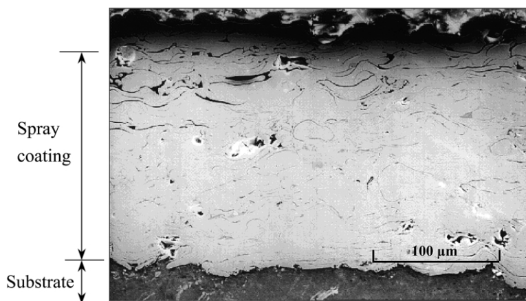
Fig. 1. Cross-section of spray coating: powder Ni-3 (Fe–2.8 C–2.1 Si–4.0 Cu–8.8 Ni–1.5 Cr–0.73 V–0.08 B).
