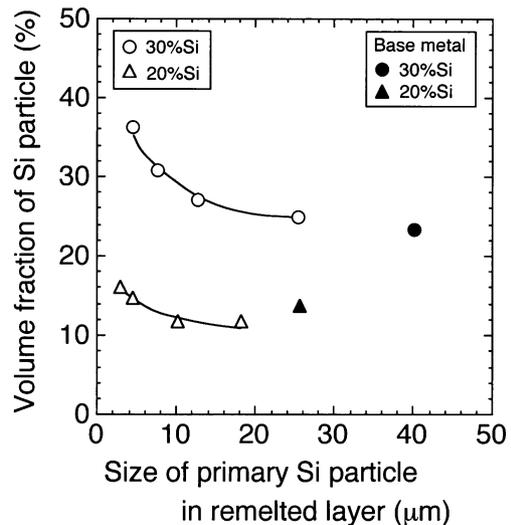
Fig. 4. Relation between primary Si particle size and volume fraction of it in the remelted layer.
