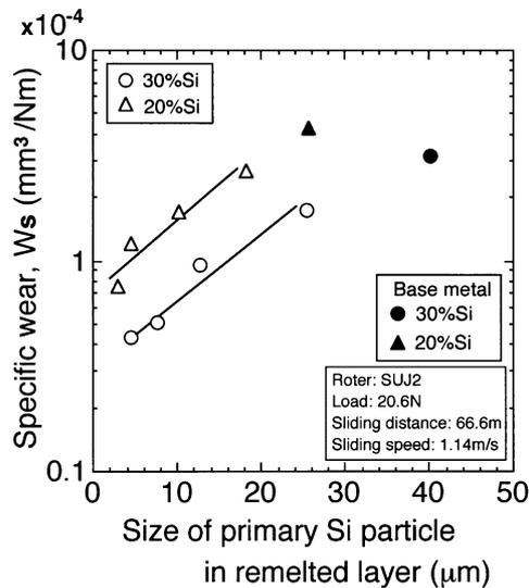
Fig. 5. Effect of primary Si size on specific wear of remelted layer measured by the Ogoshi type abrasive wear test.
