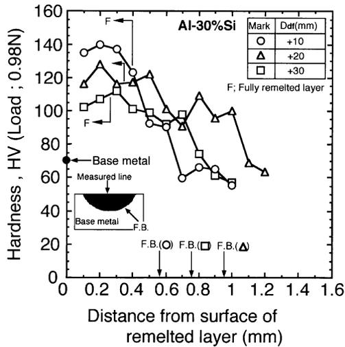
Fig. 2. Hardness distributions of remelted layers in Al-30%Si cast alloy at various defocus distance of laser beam.
