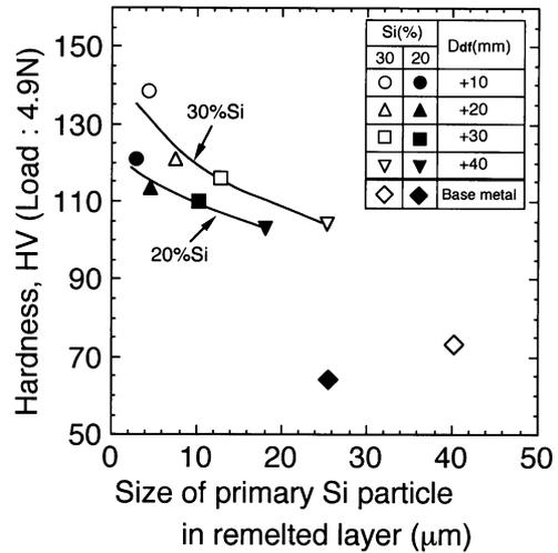
Fig. 3. Effect of primary Si particle size on hardness of fully-remelted layer.
