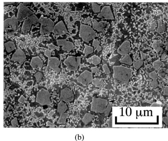
Fig. 1. Typical microstructures of cross section of laser remelted layer in Al–30% Si cast alloy. (a) Cross sectional microstructure of remelted layer at defocused distance (Ddf) of 10 mm; (b) primary Si particles within fully-remelted layer in (a). *F*; fully-remelted layer, *P*; partially-remelted layer, *BM*; as cast structure.
