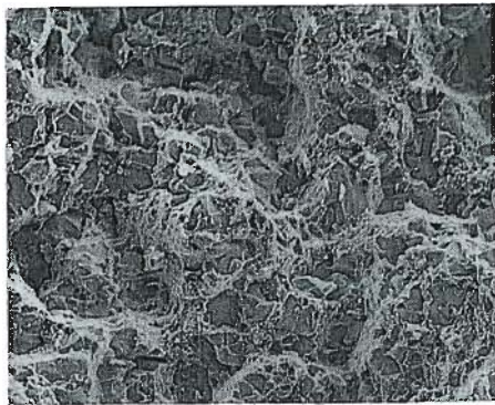
(1)-(b) Fully remelted layer by laser irradiation
