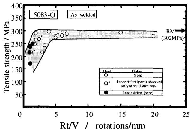
Fig. 10. Effect of welding parameter on tensile strength of FSW joint, 5083-O
