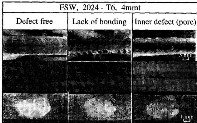
Fig. 5. Appearance and X-ray radiography of FSW joint
