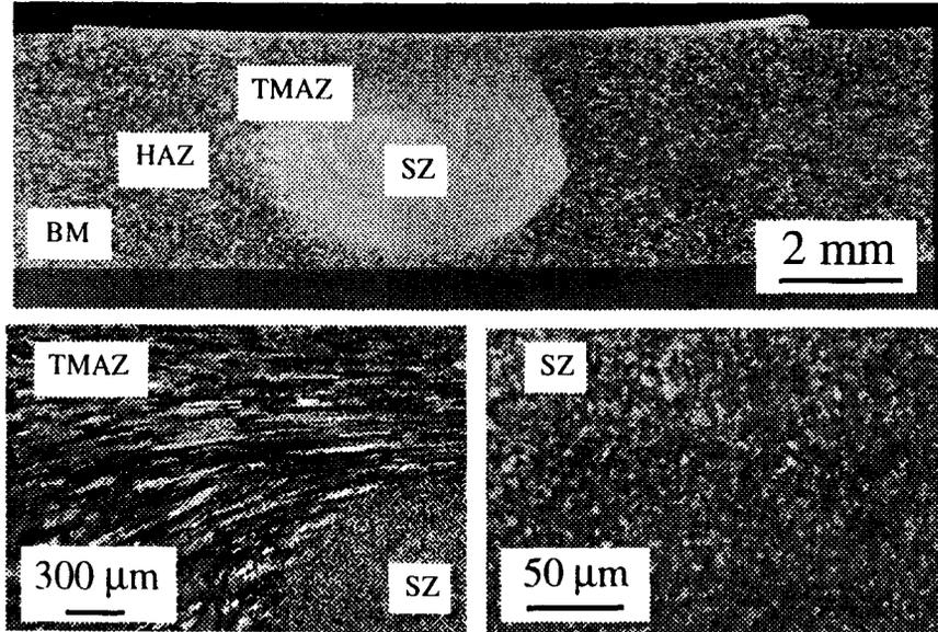
Fig. 7. Typical macro- and microstructure on cross-section of FSW joint, 2024-T6
