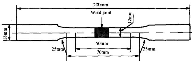
Fig. 2. Tensile test specimen geometry (JIS13B)
