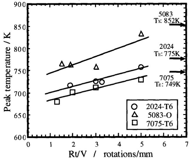
Fig. 3. Relation between welding parameter,  $R_t/V$  and peak temperature of welded joint during FSW
