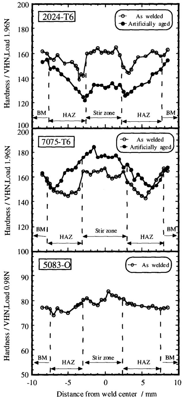
Fig. 6. Microhardness traverse on FSW joints
