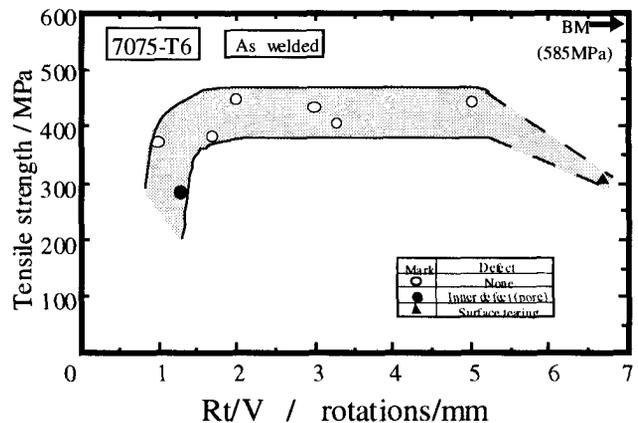
Fig. 9. Effect of welding parameter on tensile strength of FSW joint, 7075-T6
