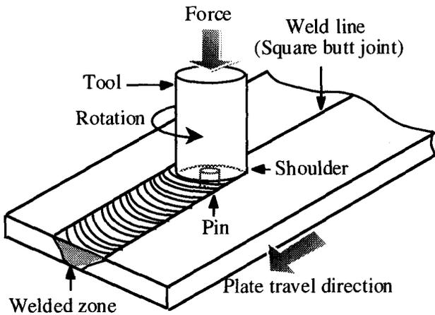
Fig. 1. Schematic illustration of friction stir welding
