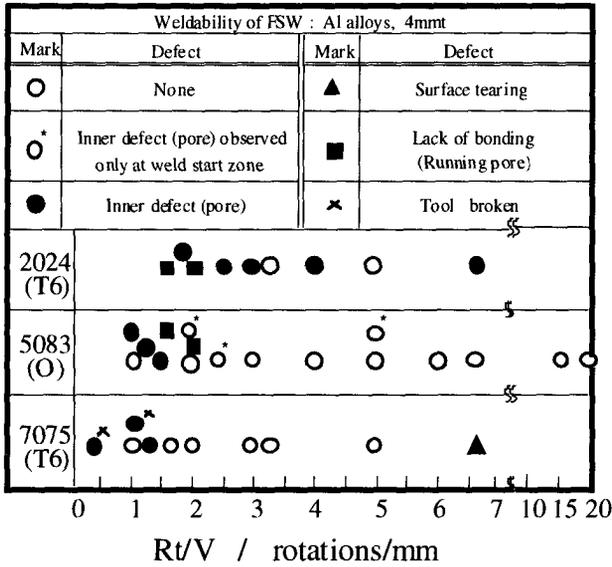
Fig. 4. Relation between welding parameter and joint quality
