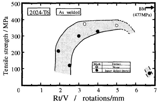
Fig. 8. Effect of welding parameter on tensile strength of FSW joint, 2024-T6
