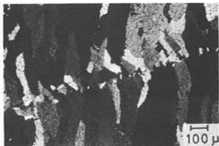
Photo. 5 Occurrence of new crystals at ripple site. material; 5052 (E), V = 250 mm/min, I = 70 A, 400 G, 2 Hz
