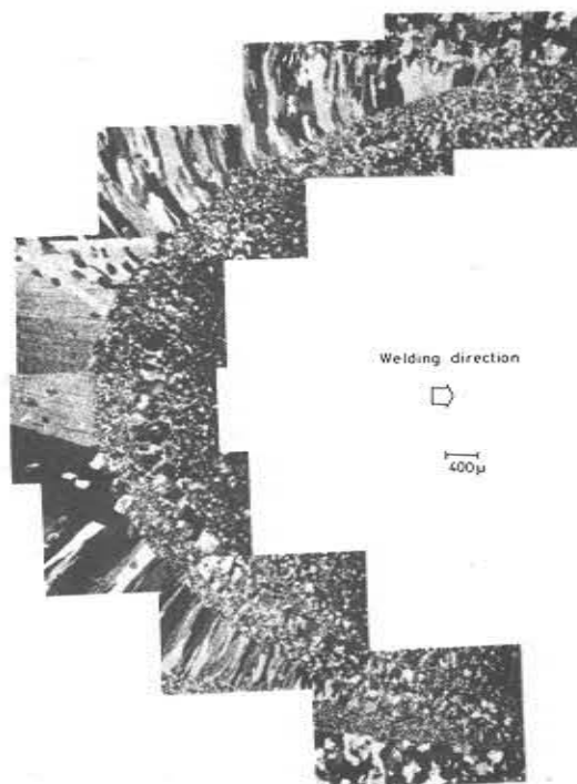
Photo. 15 Extinction of feathery crystal by application of electromagnetic stirring, material; 7N01 (K), V = 250 mm/min, I = 90 A, 5 Hz, 300 G
