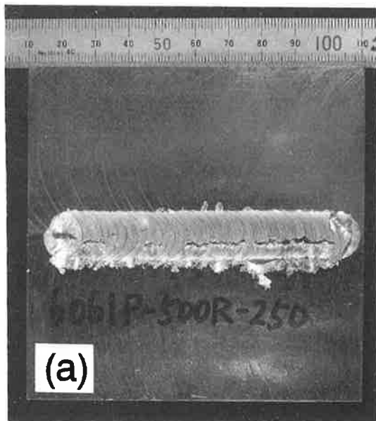
Fig. 1 Appearance of FS welds at the tool rotation speeds of 500 rpm (a) and 1000 rpm (b) with a constant welding speed of 250 mm/min.
