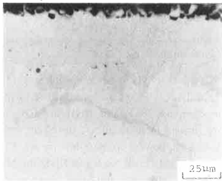
Fig. 24 Crosssectional microstructures of boronized Ni-20 Co alloy (X400).
