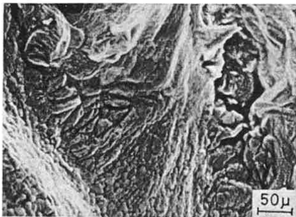
Fig. 18 SEM microstructure of irregular shaped worm hole.
