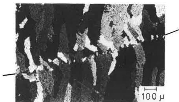
Fig. 7 Occurrence of new crystals at ripple site. material; 5052(E), V=250 mm/min, I=70 A, 400G, 2 Hz
