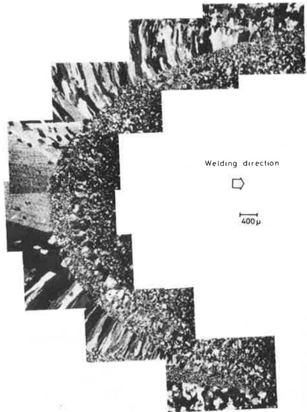
Fig. 20 Extinction of feathery crystal by application of electromagnetic stirring. material; 7N01(K), V=250 mm/min, I=90A, 5 Hz, 300G
