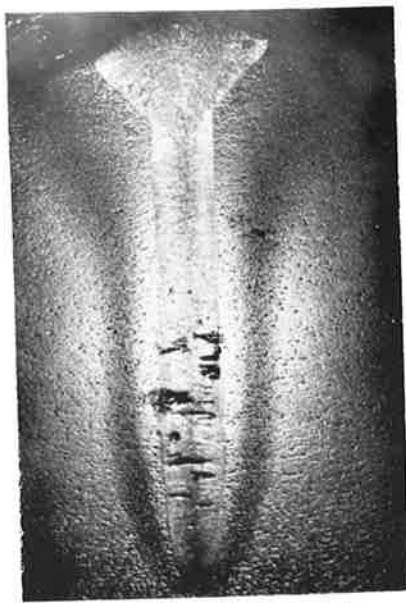
(a) Horizontal Crack (SNC2 steel) (×2.5)
