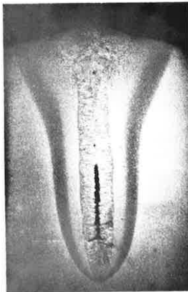
(b) Vertical Crack (I) (SNC22 steel) (×0.9)
