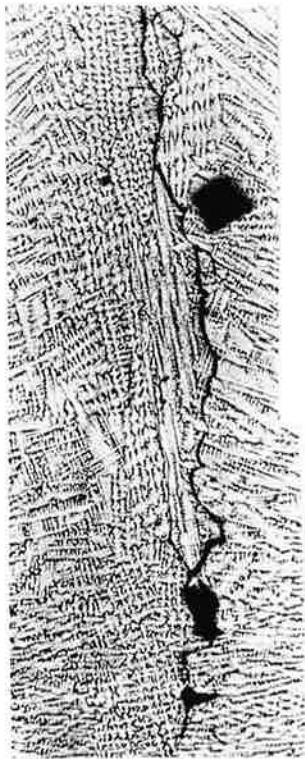
Fig. 20. Microstructure of Cracking Zone in Fig. 19 (a) (Solidification Structure) ( \times 100 ).
